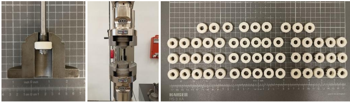
Figure 4. Sample in measuring fixture (left), Zwick Roell Z100 measuring device with sample (middle), selected 3D printed sample sets for experiment (right)
