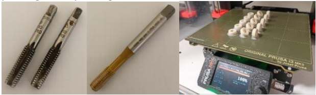
Figure 1. M10 cutting tabs (left), M10 forming tap (middle), 3D printed samples (right)
