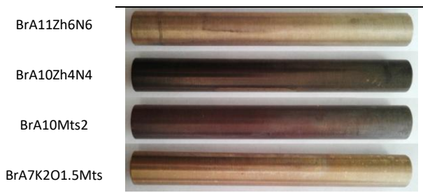
Figure 12. Appearance of the machined surfaces of “as-cast” bronze samples cast in a sand mold, after their exposure to standing seawater for 180 days
