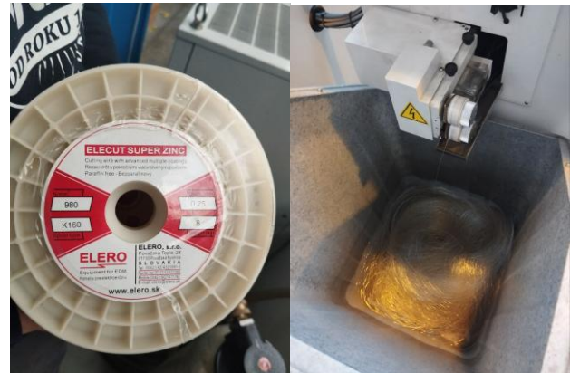
Figure 4. Cutting wire Ø0.25 mm with the Elecut Super Zinc marking used in WEDM of F10 and G30 sintered carbides
