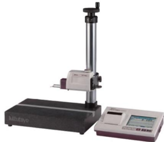
Figure 2. Mitutoyo SJ 400 contact roughness tester used in the experiment
