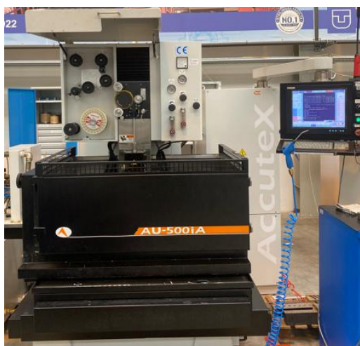
Figure 1. Accutex AU-500iA EDM machine from Accutex Technologies Co., Ltd. used to produce experimental samples
