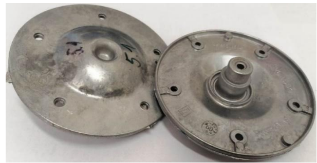
Figure 2. The electric motor flange cast
