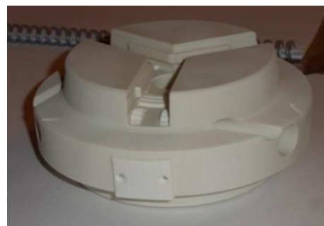
Figure 6. Model of the assembly lathe chuck produced by additive technology SLS. [Bulira 2017].
