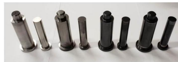
Figure 3. Uncoated punches and punches with FeinAl, FeinAl + Movic, and Movic coatings used in the experiment
