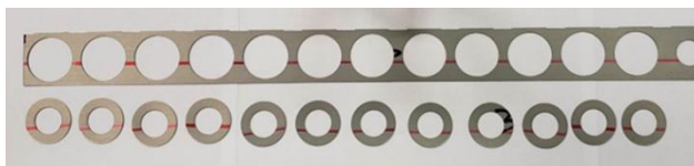
Figure 2. Annular blanks produced from material G
