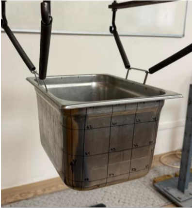
FIGURE 2 MOUNTING OF GN CONTAINER WITH MEASUREMENT GRID TO TEST FRAME.
