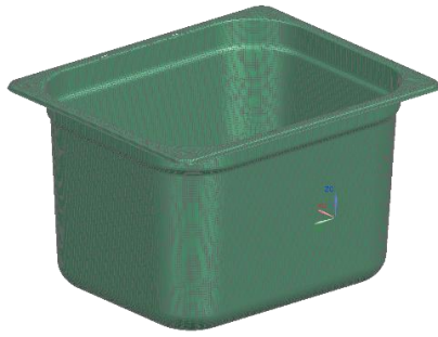
FIGURE 3 FINITE ELEMENT MESH OF GN CONTAINER.
