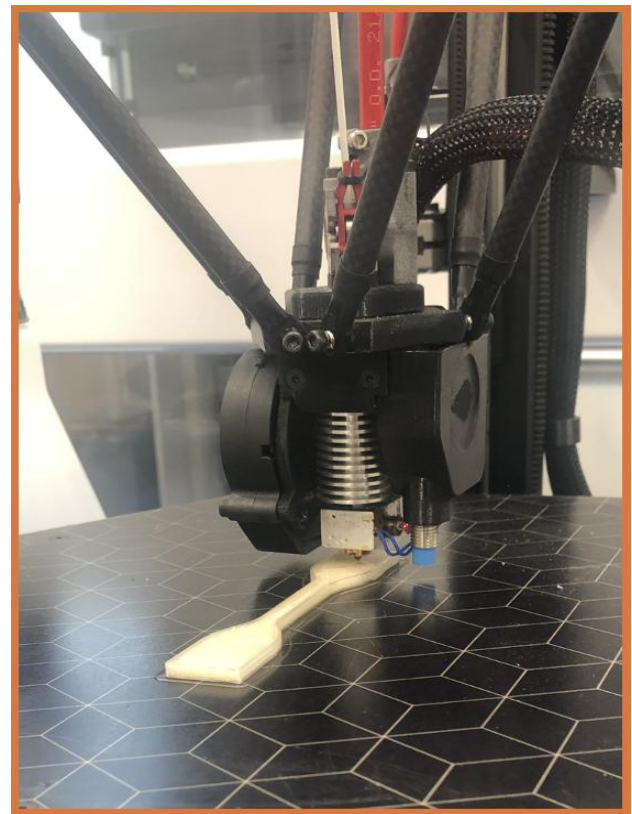
Figure 3. 3D printing process of dogbone
