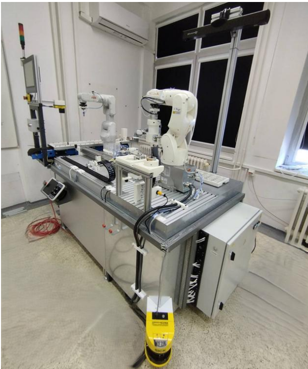
Figure 2. Experimental robotic workstation integrating ABB and KUKA industrial robots within a PLC-based control architecture.
