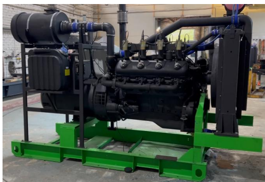
Figure 1. External view of a diesel generator set in an open-frame design
